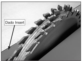
Figure 4. Dado blades installed in table saw.
